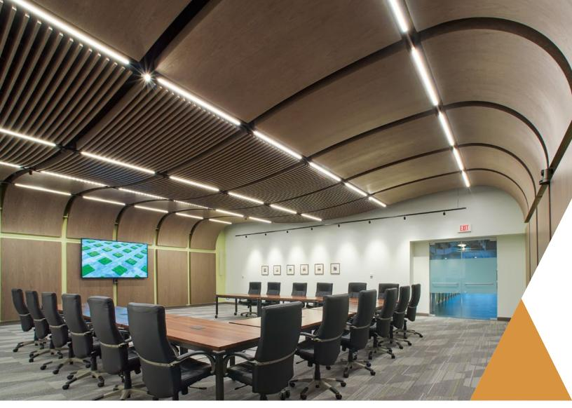
WoodWorks® custom microperforated ceiling and wall panels and Grille panels; Armstrong Campus, Lancaster, PA
