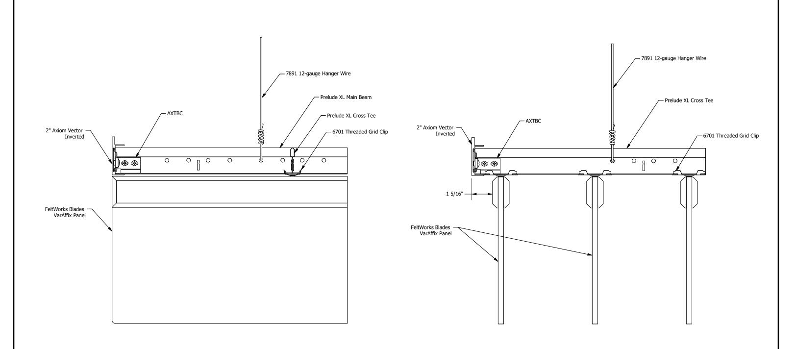
FeltWorks Blades VarAffix Floating Perimeter Details - Threaded Grid Clip Installation
