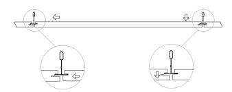
4. Gently push up on the two non-supporting edges at the location of the Mid-Point Clip to engage the clip on the grid flange.
