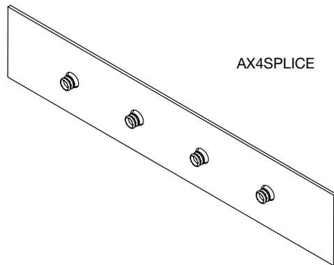
**NOTE:** Splice plates can slide completely into the channel bosses and then slide into the adjoining section after the cove is aligned. This aids splice plate connections for the last piece.
