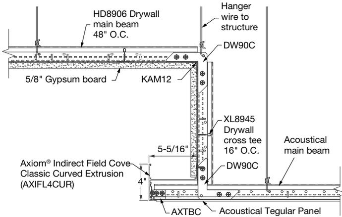
Axiom® Indirect Field Light Cove corners can be ordered in both Knife Edge® and Classic trim for both the ceiling-to-wall and the ceiling-to-ceiling coves. Pre-made factory-finished inside and outside corners are made to coordinate with the straight Indirect Field Light Cove sections. Each corner section is 12" by 12" square (dimension taken on the face of the extrusion).
