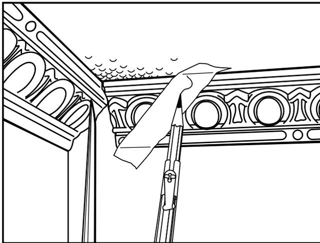
Cut along the scribed line and test fit the coped cut. You may have to make some minor trim cuts to make the parts fit. Once the coped end fits, you can use it as a template to mark a length of cornice for installation. If you are using bare steel cornices that will be painted, you can use putty to fill in any bad fitting joints.
