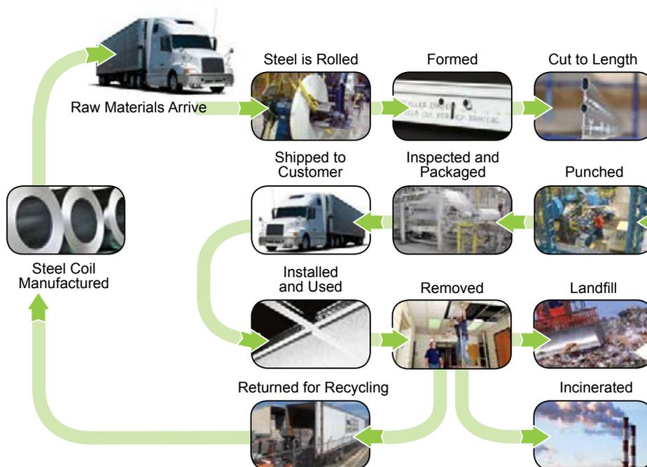
Armstrong® suspension systems use hot dipped galvanized steel which is formed into coils. A large component of the steel is recycled material. The coils are split and painted, and then sent to Armstrong World Industries. At the Armstrong Ceilings plant, the steel is pressed, roll formed, punched, and packaged. The material is then shipped and installed. When the system is disassembled, the majority of the steel is recycled.
