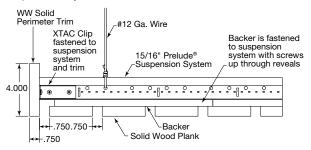
Perimeter trim installed on the border at panel ends, perpendicular to the suspension system, should be installed by using a mechanical fastener to secure 7800 wall molding to the suspension system and trim.
