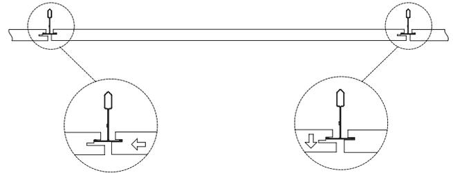
**STEP 3:** Slide the panel so that the registration kerf on edge "B" engages the grid flange. Ensure that the access kerf on edge "A" drops down into the correct position.
