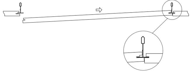
**STEP 2:** Raise the "B" edge of the panel, the registration kerf, into the grid opening until the kerf lines up with the grid flange.
