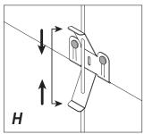
STEP 6: Turn all hooks in the same direction, parallel to joists. Set all hooks to about the same height.
