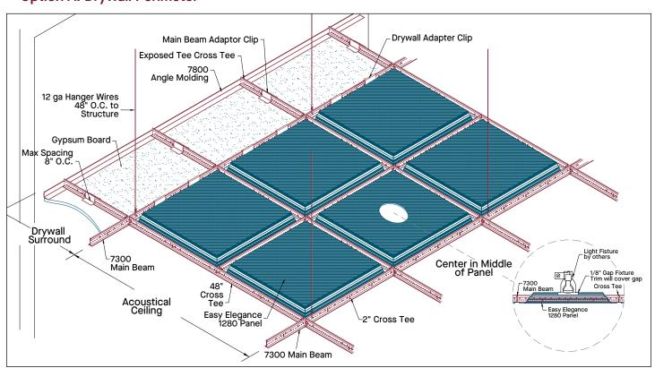
Parts needed: 7300 Prelude® Main Beams and coordinating Cross Tees, MBAC Clip, DWAC Clip, and CHDC Clear Hold down Clip, 1280 or 1282, 1/2" or 5/8" drywall, angle molding, hanger wires and wire fasteners, square edge drywall casing bead (J-channel), Type S 1-1/4" screws, spackle, drywall tape, and paint.
