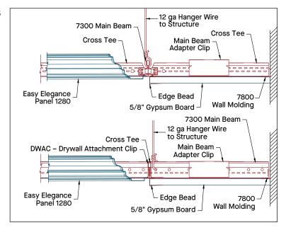
Parts needed: Easy Elegance Flat panels, and 1280 or 1282 Coffered panels, 7300 Prelude Main Beams and coordinating tees, CHDC Clear Hold Down Clips, angle molding, hanger wires and wire fasteners.
