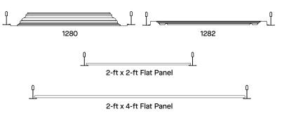
**Lighting:** Easy Elegance panels work with most modern light fixtures. Leave a 1/8-in gap between recessed light housing and panel. Additionally, the 1280 panel is 2.5-in tall, so light fixtures may require a height extension component to provide clearance above the panel when installed. Consult local electrical code or lighting fixture manufacturer for all light fixture requirements.
