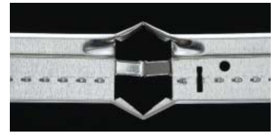
Main beam exposed to fire
