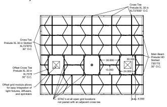
For 2' x 2' grid layouts and panels consider placing lights, diffusers, sprinklers, etc. into square panels throughout the pattern. Example: Patterns TS-0003.
