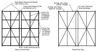
Back view - lighting integration in 6" technical zone perpendicular to main beams
