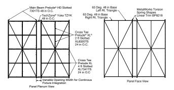
The trim is designed for use with continuous linear fixture openings that run parallel to the main beam direction, and are framed with mains. An optional layer of foam tape (gasket) can be applied to the trim, if desired. The trim is screw-attached to grid that frames the linear opening and is only compatible with full-size panels.
