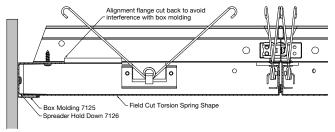
For perimeters using Axiom trim, the Axiom Serpentina Hold Down Clip (AXSPTHDC) must be used. Install as needed to ensure that the cut panel face is tight against the flange of the trim.
