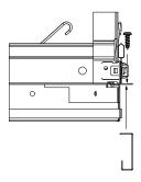
2. Use 1/2" sharp point metal framing screws (provided by contractor) to fasten the trim to the grid no more than 24" O.C. and within 8" of each end of the trim. If the fixture will interface with the grid flange then the trim must be screwed from the top down.
