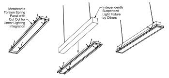
**8.2.2.2** Pendant lights are also able to be used at the intersections of panels. The electrical cord must be wrapped in foam at any locations that could come into contact with metal panel for safety precautions. The light also must be independently supported.
