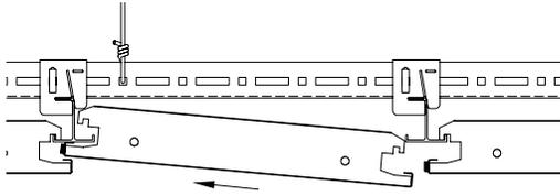
**Step 1:** Fully insert the left side of panel above adjacent panel.
