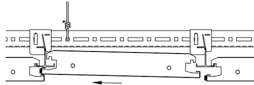
**Step 2:** Slide desired panel for removal to the left. Slide panel face into gap below 1-bar of adjacent MetalWorks panel (careful not to scratch panel face). Be sure that the corner hook-on left of MetalWorks panel is clear of 1-Bar.
