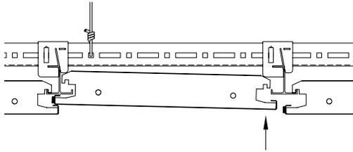
**Step 2:** Raise right side of panel so the corner hook is above the 1-Bar.
