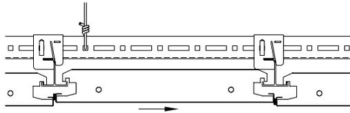
**Step 3:** Slide RH215 panel to the right until the corner hook is over top of the 1-Bar.
