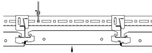
**Step 1:** Carefully lift panel evenly so that the corner hook disengages the 1-Bar.
