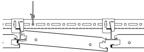
**Step 3:** Lower right side of MetalWorks panel below the bottom edge of 1-Bar.
