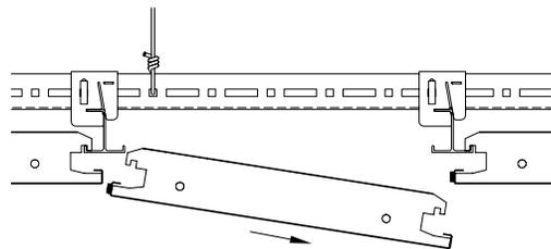
**Step 4:** Slide MetalWorks panel to right past the bottom of 1-Bar on left. Lower panel past 1-bar on left. Make sure panel clears 1-Bar carefully.
