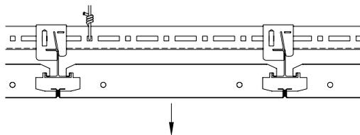
**Step 4:** Lower MetalWorks panel evenly onto 1-Bar. Check panel(s) for proper alignment.
