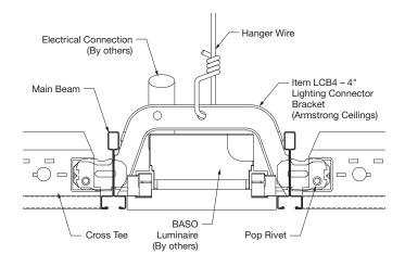
Below is an overview of the ceiling system components required to complete one of the described on-center ceiling layouts.
