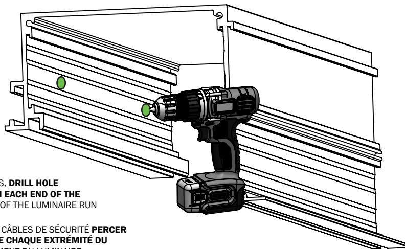
TO INSTALL SAFETY CABLES, DRILL HOLE APPROXIMATELY 8" FROM EACH END OF THE LUMINAIRE OR SEGMENT OF THE LUMINAIRE RUN
