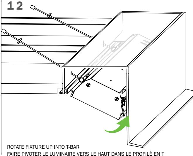
ROTATE FIXTURE UP INTO T-BAR
