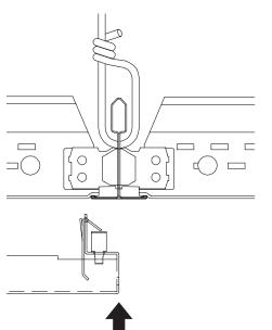
Lift panel to suspension system flange
