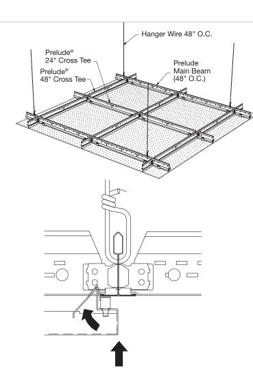
Gravity clip rotates to clear suspension system flange
