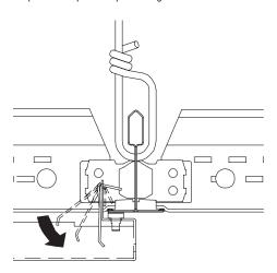
Gravity clip rotates back down after suspension system flange is cleared (spring is compressed)
