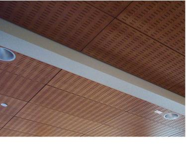
Flat Panel Series 7 (SS7) is available in standard and custom sizes up to 3ft wide and 10ft long to meet particular design requirements. Special surface patterns and logos can also be incorporated into the manufacture of the panels. Perforation options control sound absorption, and acoustic insulation is added behind panels for greater NRC performance. Acoustical fabric is attached to the back of the perforated panels to increase acoustical absorption.
