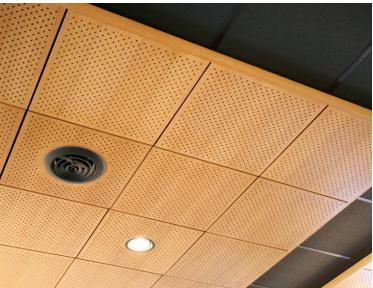
Flat Panel Series 4 (SS4) is a ceiling panel system with a wood backer suspension to hang below the Armstrong® Prelude® XL® grid to create 3/8" reveal between panels. Panels incorporate a lift and shift for accessibility.
