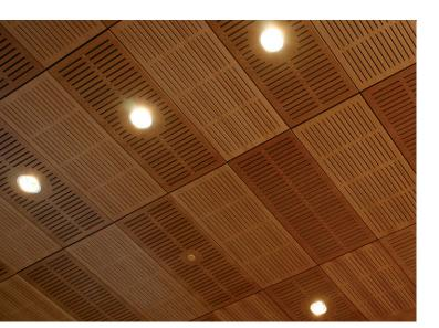
Flat Panel Series 3 (SS3) is a ceiling panel system with a reveal edge suspension to hang below the Armstrong® Prelude® XL® grid to create 3/8" reveal between panels. Panels incorporate a lift and shift for accessibility.
