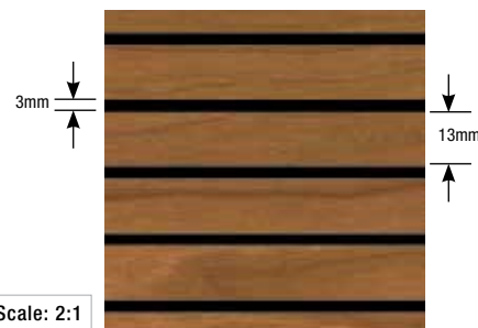
W7 Type: Channeled Groove Size: 13mm profile with 3mm groove
