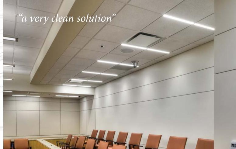
"Aesthetically, the T-BAR LEDs provided a very clean solution. Functionally, they allow speakers to be positioned based on where they are best suited. And to top it off, the various ducts, sprinkler pipes, and electrical conduits easily fit without having to coordinate around light locations."
