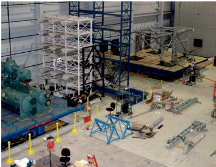
SEESL's twin relocatable shake tables
