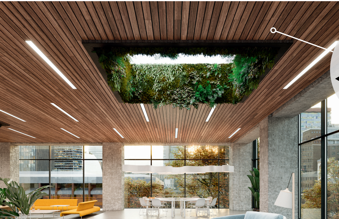
WoodWorks® Linear Veneered Open 3-3/4" planks in Plain Slice Walnut (NWN)
