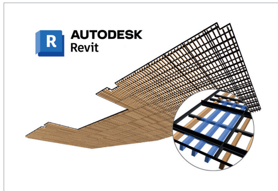
Revit models can be imported into building models and contain detailed panel and suspension data to accelerate the design process.
