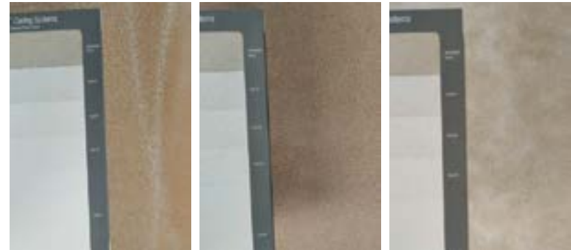
Low Pressure (Spray pressure is too low)
